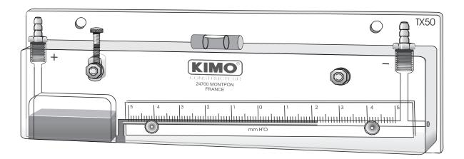
The TX range of inclined liquid column manometers, developed and manufactured by KIMO, measure slight variations in pressure, depression or differential pressure.
